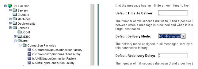
Then Navigate to Services==> JMS==> ConnectionFactories ==> CICommonTopicConnectionFactory and double click and Change Default Delivery Mode to NON-Persistent
